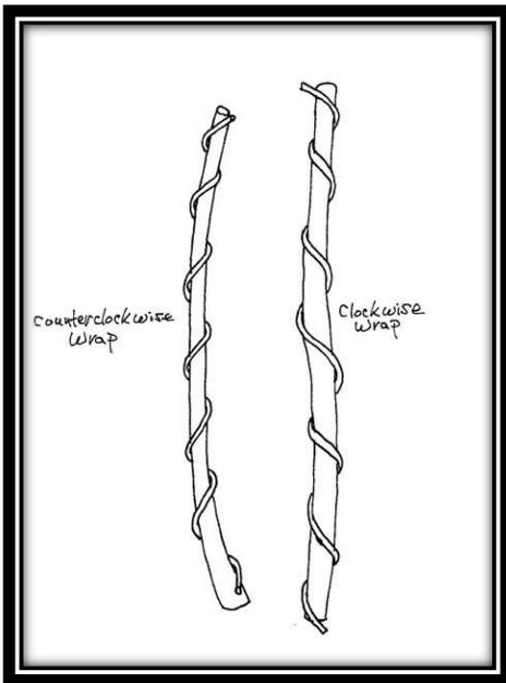
Figure 1(left): To convince yourself that these wraps are fundamentally different, study this diagram, but to make the experience really meaningful, get your own sticks and some wire thick enough to hold a bend in them. Wrap one stick clockwise and the other counterclockwise then experiment with bending these wired sticks
